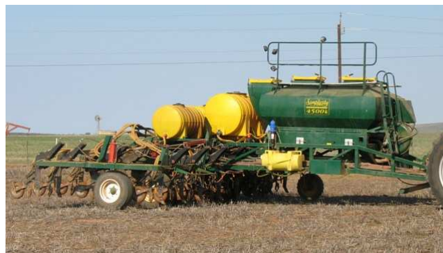
Picture 1 - Minimum till planter rigged with two 500L tanks for Compost Tea and a 100L tank with Dosatron pump for the Apex.
