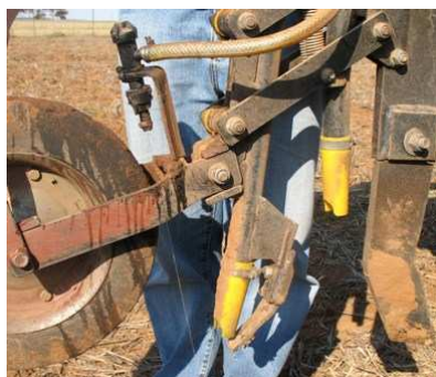
Picture 3 - Compost Tea and Apex is dosed directly onto the seed as it is planted. The thin jet of Compost Tea can be seen just left from the yellow seed nozzle. The yellow nozzle on the right is for fertiliser application
