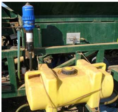
Picture 2 - Dosatron pump set at 10% with 100 L tank for the dosing of the Apex
