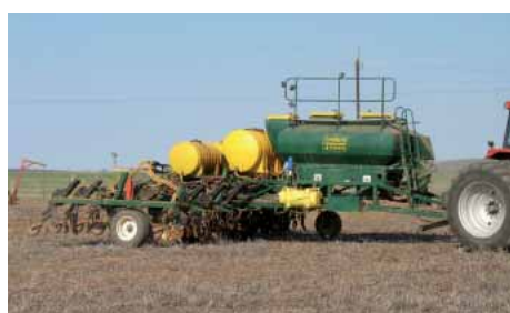
Wheat planter with 1000L tank for compost tea. The compost tea is pumped out by a diaphragm pump.
