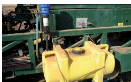
The Apex is administered from a separate tank with a dosatron pump.
